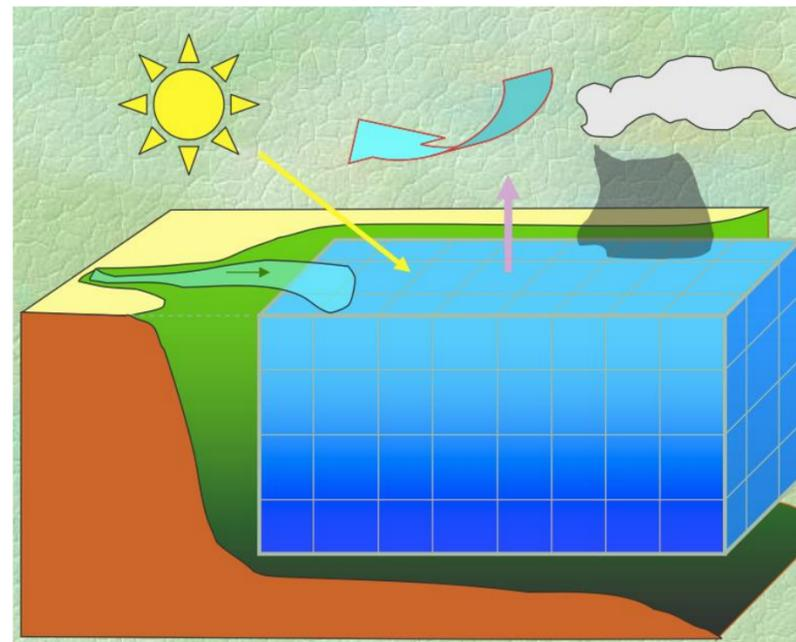
Computational grid: the equation are discretised in each cell considering the contribution of the surrounding cells
