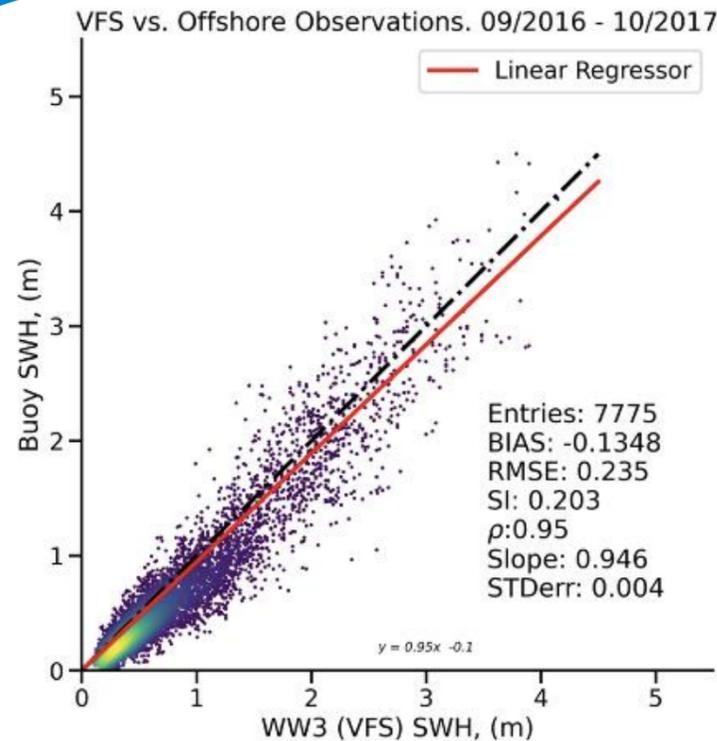
Wave model validation vs buoy
