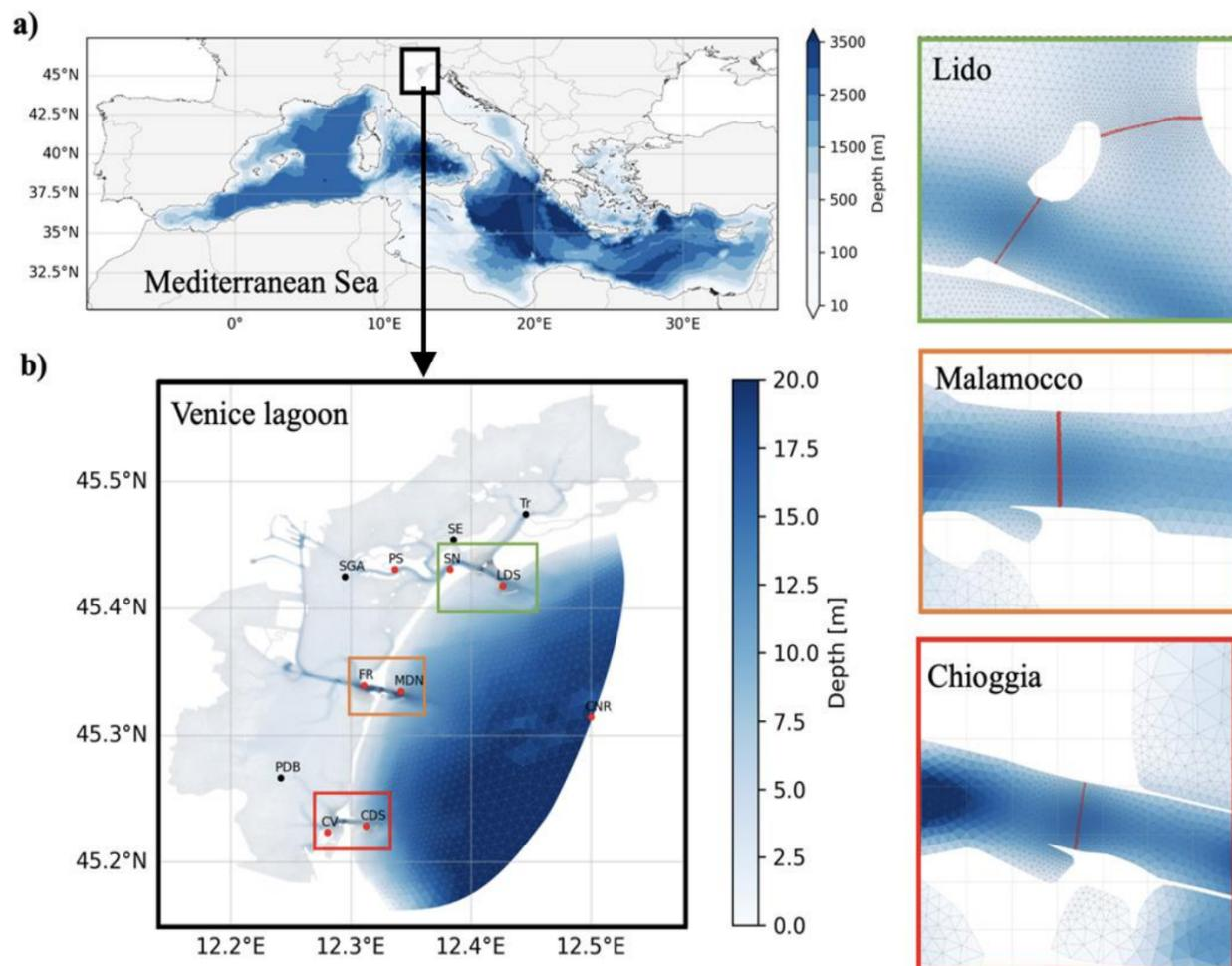
Immersed boundary condition developed in SHYFEM-MPI for simulating the MoSE
