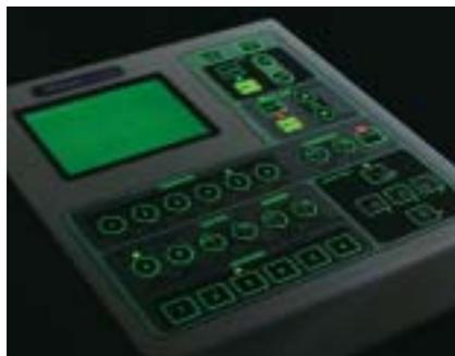
Remote control pad and filter turret use phosphorescent display tags to enhance visibility during operation in dark rooms.
