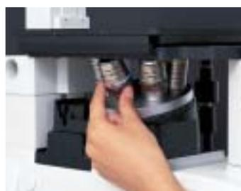
Nosepiece is inclined to the left for easy handling.
