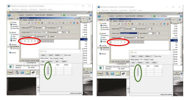
Now all the values have been changed, but on the victim's display nothing happened. The Master's display keep showing the same values (in the red oval), because now it has been connected to the fake PLC which was set with the old values. While on the actual PLC (the green oval) the values have changed.
