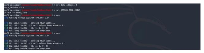
There are 5 holding registers, with the values (in order) 11,22,33,44,55 and 5 coils, with the values 1,1,1,0,0.
