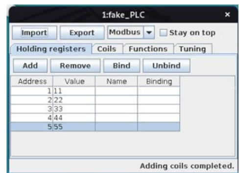
After that, the SlaveIP is changed on a new INI file with the attacker's IP (that is where the new fake PLC resides).
