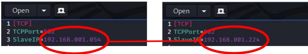
The Master software is forced-closed on the victim's system and the new "corrupted" configuration file with the new IP is uploaded to the folder to replace the current, original qModMaster.ini file.
