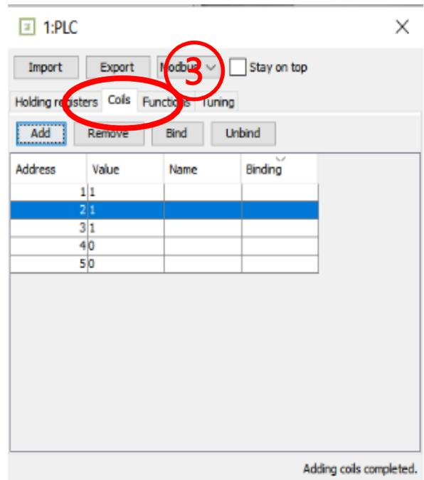
Then the connection from the Master is established by setting the IP address(5) from “Options” and pushing the “Connect” (6) button. The TCP port is left as 502, the default one. Slave Addr is the ID associated with the slave and the number of coils are set to 5. Actions are performed from the “function code” list and executed with the Read/Write button (7). In the image the function is “Read coils” and will display the coils as being set.
