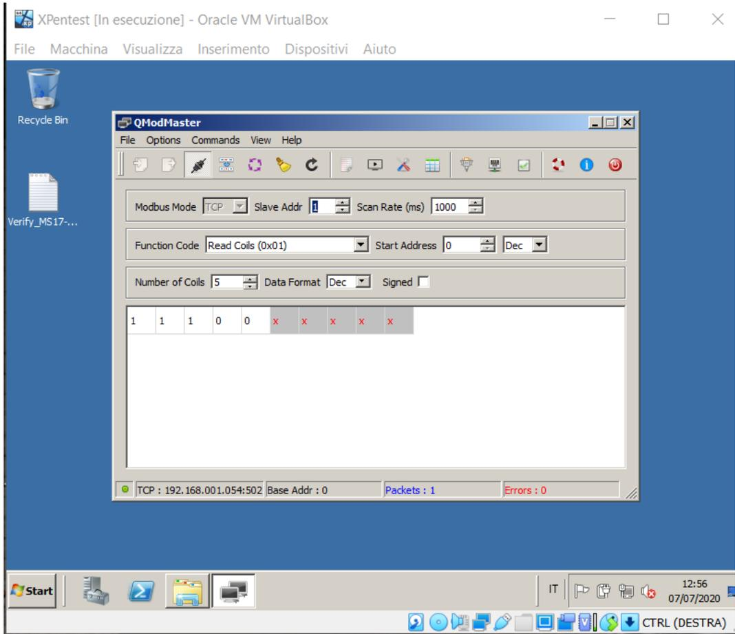
Now that the SCADA-like software is known (qModMaster), it is time to get the IP address of the slave (i.e. the PLC) in order to proceed with the attack. There are several ways to do that, depending on the context. A software like Wireshark could be used to capture the data packets that the Master and slave send to each other. Another way is to “look around” in the qModMaster’s directory and look for useful information. To do that, a shell is opened.
